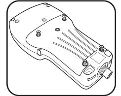
**A** CAUTION: Overtightening of the screws is likely to cause damage and require replacement of the battery pack.
